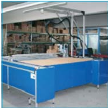
Bickers-JMP GLUEJET® XY-Glueing Table standard with 4 independent work stations
